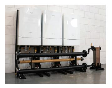
When specifying a low loss header, make sure it is sized appropriately for the boilers you are going to use it with and your expected flow rates. If the flow velocity in the body of the header isn't low enough, you won't get effective separation between the two systems.
