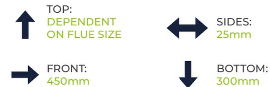
CLEARANCE BETWEEN MULTIPLE BOILER INSTALLATIONS: 25mm
