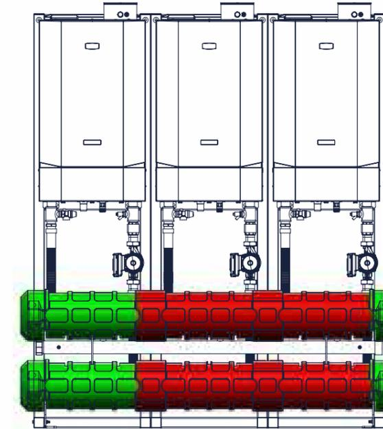
STANDARD HEIGHT INSULATION STARTER KIT + STANDARD HEIGHT INSULATION CONTINUATION KIT + STANDARD HEIGHT INSULATION CONTINUATION KIT
