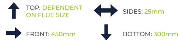
CLEARANCE BETWEEN MULTIPLE BOILER INSTALLATIONS: 25mm
