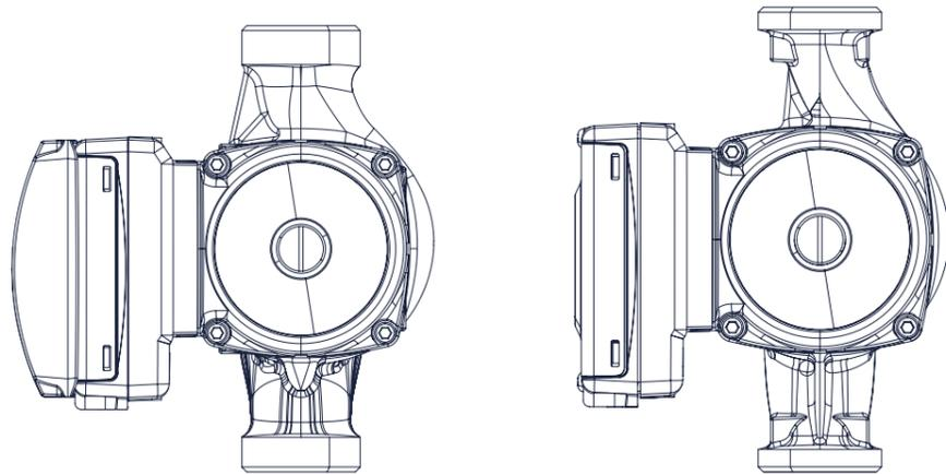
Note: pumps with screwed connections are G1.1/2" x 180mm.
