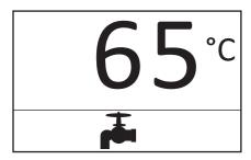
Now press the + or - button to set the desired HW temperature.
