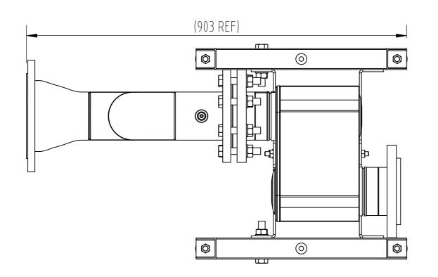
Note 1: Plate Heat Exchanger and gas connections can be located either on the LHS or RHS of the assembly to suit the needs of each particular system.
