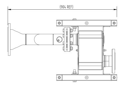
Note 1: Plate Heat Exchanger and gas connections can be located either on the LHS or RHS of the assembly to suit the needs of each particular system.
