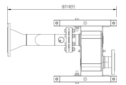
Note 1: Plate Heat Exchanger and gas connections can be located either on the LHS or RHS of the assembly to suit the needs of each particular system.
