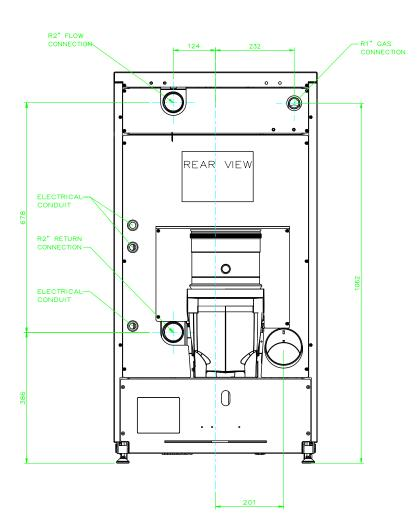
THIS DRAWING COVERS 200kW, 240kW AND 280kW BOILERS
