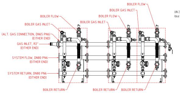
UIN 226402, IMAX XTRA 2, 3 BOILER HEADER KIT, 80–120kW, DN80 PN6 WATER, R2" TO DN65 PN6 GAS, THREADED PUMP Ideal Heating reserves the right to amend details or specification without notice. If in doubt please contact an authorised representative
